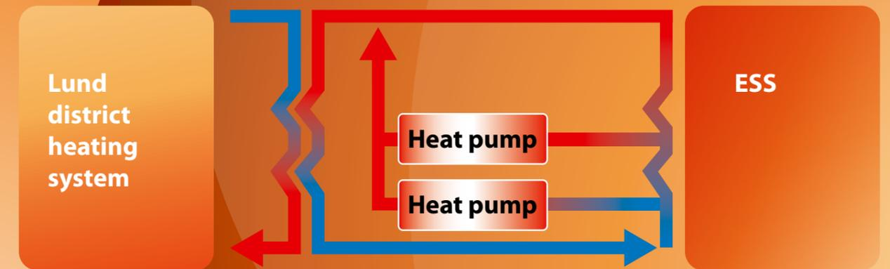
THE FLOW OF HEAT FROM ESS TO A DISTRICT HEATING SYSTEM.
